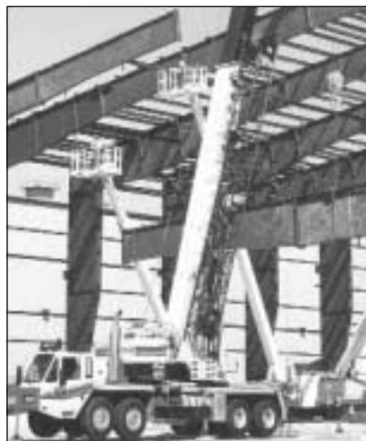
A Link-Belt HTC-8660 60-ton hydraulic truck crane with the new air-ride suspension.
