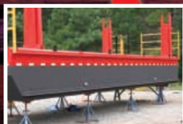
Towable, sectional jack-up barges.
