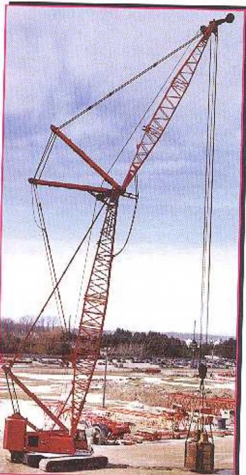
The new No. 149 high-capacity luffing jib was recently introduced by Manitowoc Cranes.
