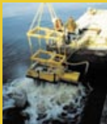
PRIME® WATERJET ATTACHMENT 24" Cutter with Waterjet Attachment for cutting below mudline
