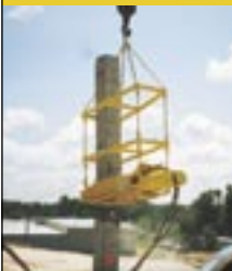
PRIME® PILE CUTTER 16" Cutter with 2-Part Cradle
