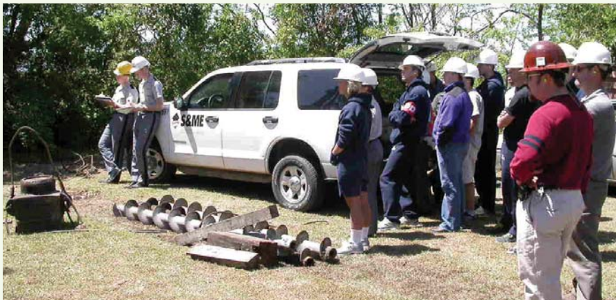
Citadel students record blow counts and gather around Greg Canivan to watch the pile driving and observe his PDA analysis.
