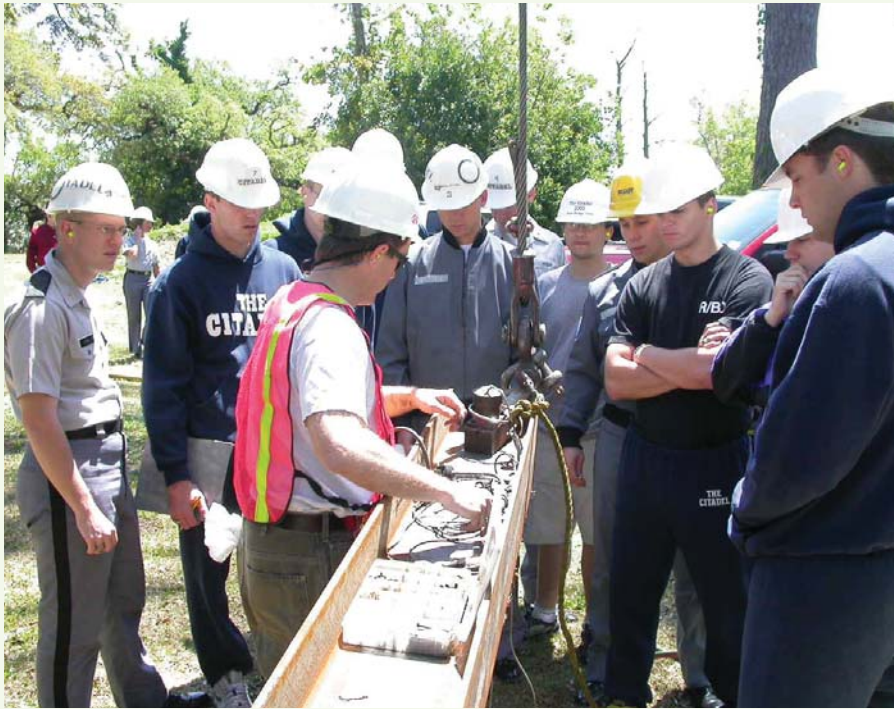
Greg Canivan of S&ME demonstrates how strain gages and accelerometers are attached to a steel H-pile.
