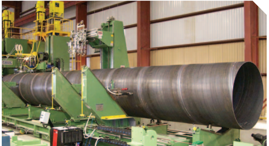
60-inch Trinity Lo-Profile Spiral Weld Steel Pipe being welded. The piles have received a favorable review from the U.S. Army Corps of Engineers' Innovation Team.
