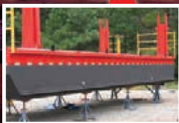
Towable, sectional jack-up barges.
