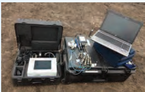
Figure 3 – Wireless and remote capabilities of PDI’s PAX
