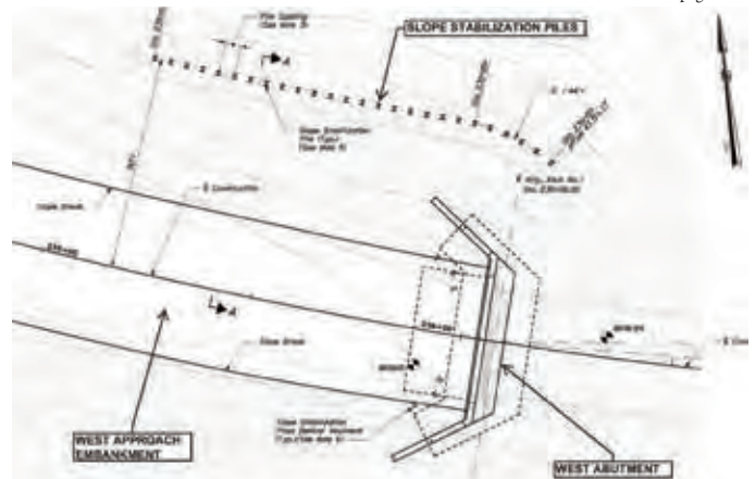
Plan limits of HP12x53, slope stabilization piles along the north side of the west approach embankment and behind the west abutment
