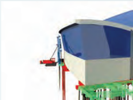
Fig. 5. BIM model of the rig in driving position on the south side of the terminal
