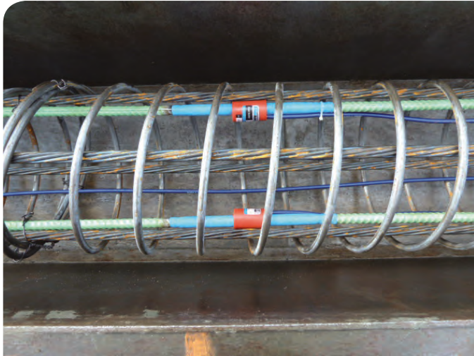
Rebar strain gages in LW50 pile
