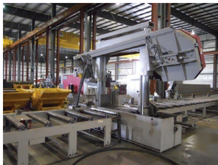
Laser-guided automatic feed band saw in the Columbia City, Ind. warehouse
