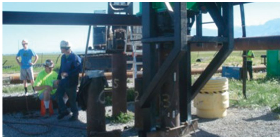
Plate 1: The instrumented 2003 pile under the IP3 hydraulic hammer
