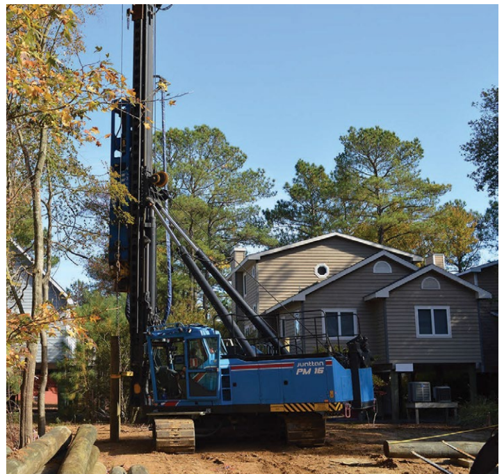
PM16 with 4 ton hammer
