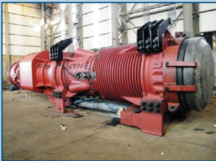
The new D800-12 diesel hammer for large-diameter monopiles
