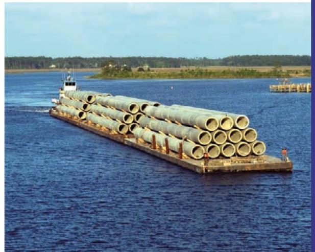
Piles Produced in basic 16 ft sections with 4 ft, 8 ft and 12 ft available
