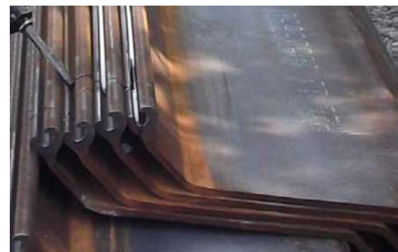
Steel sheet pile locks filled or being filled with sealant
